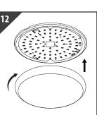
Push and twist the diffuser back into place
