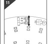
Use the CCT selection switch on the gear tray to select the desired colour temperature
